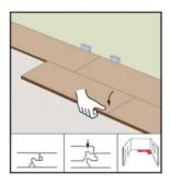
when they meet the new panel can be lowered to the sub floor to lock it into position, apply pressure to the head joint to complete the joint
