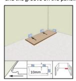
Begin installing the first row from the Right-hand corner of the room with both tongue sides of the panels pointing towards the wall. Place spacers between the edges of the flooring panels and the walls to provide the correct space for expansion.
