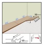
The second row is started by using the off cut from the previous row if it's greater than 200mm, at an angle place the tongue edge to the groove edge of the first row, don't forget to allow for expansion at the beginning of the second row, once located the new panel of the second row can be lowered to the sub floor locking the newly formed joint.
