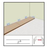
Continue with this method until the end of the first row. Mark the last panel in the first row to the required length (place tongue to tongue) and cut.
