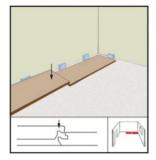
Connect the second panel to the first by placing the interlocking end of the new panel from above and press down to form the joint between the boards.
