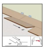
The second panel is located in the groove of the first row in the same way, once located the second panel can be slid towards the first panel of this row.
